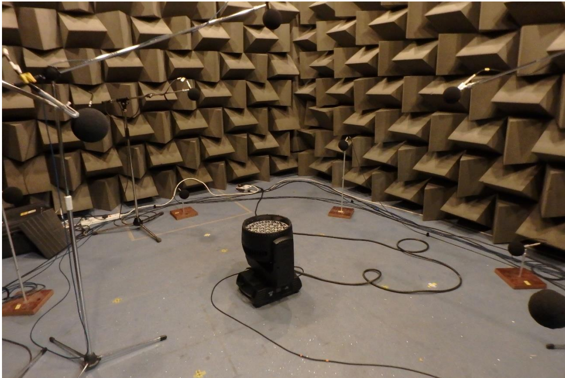
Figure 1 – unit under test mounted in the hemi-anechoic chamber at the University of Salford.
