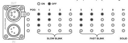
If all indicators on a pod are on and not blinking, that pod exceeds the capacity of the connected driver and will not function
