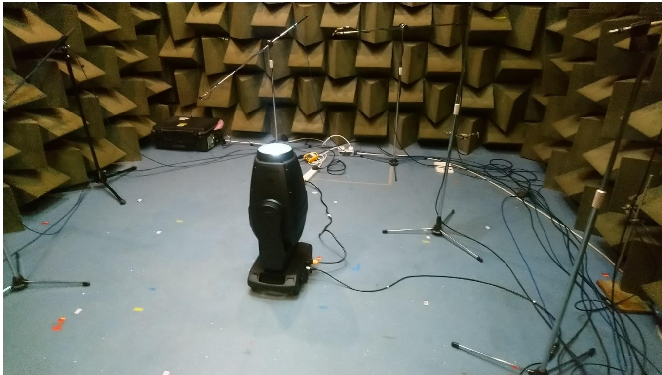
Figure 1 – unit under test mounted in the hemi-anechoic chamber at the University of Salford.
