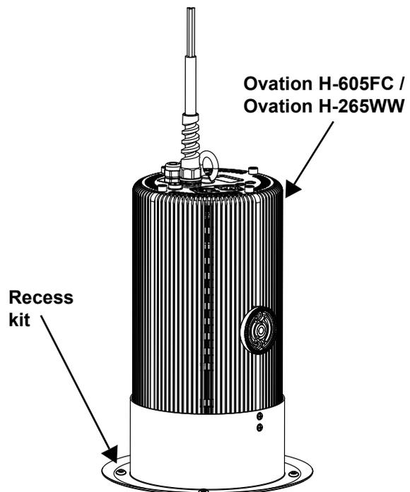
4. Attach the fixture into the ceiling using 4 pieces of M4 screws.
