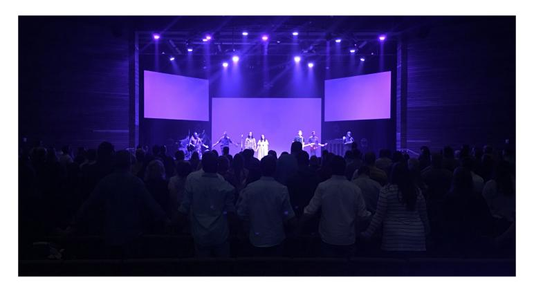
Harris Creek Baptist has seven Maverick MK2 Wash fixtures, 16 Rogue R2 Wash fixtures and 10 Rogue R2X Spot units. Positioned across the front bar, the Maverick fixtures are used for key lighting or soft spots during worship. The versatile RGBW fixture with a 7° – 49° zoom range is also used for color saturation and as a side light during preaching to soften the coverage from the rig's ellipsoidal units.
