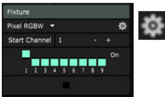
12. Existing fixtures may be modified and new fixtures may be added in this window. They can be renamed in order to help identify them in the **Advanced Output** window.
