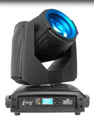
Legend™ 230SR Beam features a 230 W Osram Sirius lamp outputting an intense 96,000 lux at 15 meters, thanks to precision glass optics and a tiny 2.25° beam angle. Compact and agile, it also features a zooming 8-facet prism and 17 gobos (plus open) for beam shaping effects, along with automated focus. In addition to 14 solid colors plus white, the color wheel delivers seamless split colors.
