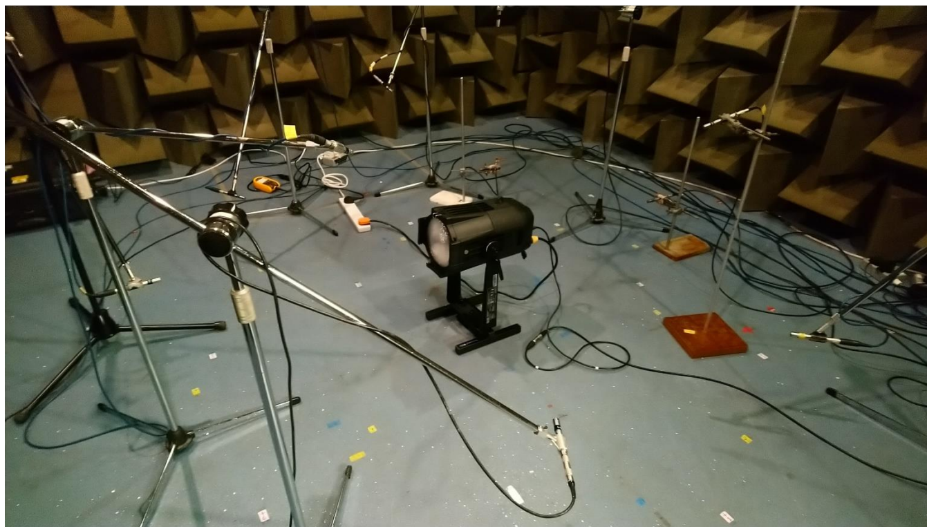
Figure 2.1 – Example of the typical arrangement of a unit under test, as mounted in the hemi-anechoic chamber at the University of Salford. (N.B. this image does not represent the specific unit covered by this Test Report.)
